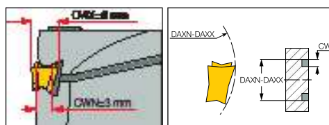
Insert initial face grooving range
